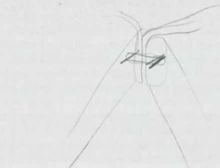
5b Sketch by Ronan Bouroullec showing one way in which to assemble the chair using wooden dowels. At one stage they considered an H-shaped construction featuring three dowels, one more than they used for the definitive design.
