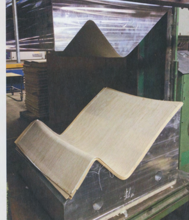
6 Here the seat, made up of several layers of veneer interleaved with fabric, is ready to be pressed into the mould and shaped.
